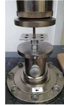
Figure 3. The set-up for push-out tests
