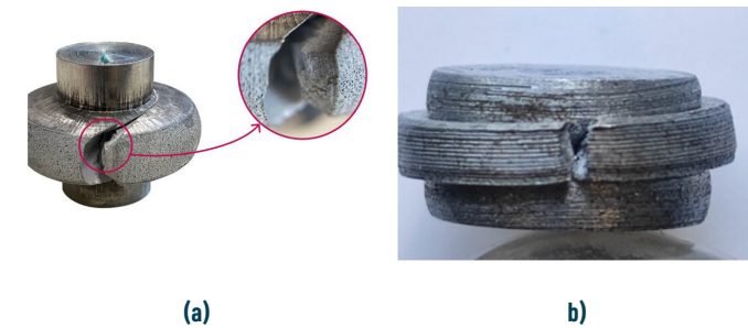
Fig. 6 Images of cracks obtained with center flange geometries (a) AA6082 [13] (b) C45E Image (a) adapted from [Rui F.V. Sampaio et al.,2023, On the utilization of radial extrusion to characterize fracture forming limits. Part II: testing and modelling, Materials Research Proceedings]. Used with permission.
