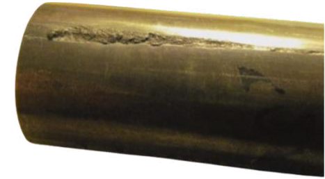
Figure 2. Cylinder that galled on removal from a conforming cylinder [20]
