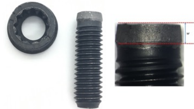
Fig. 4. Specimen that fractured after tensile tests.
