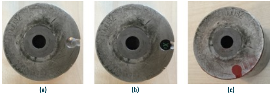
Fig. 1. RFID tag assembly steps: (a) Opening the assembly slot, (b) placing the tag, and (c) sealing with a liquid gasket.
