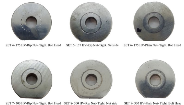
Figure 9. Plate deformation caused by rip form during different tightening strategies.
