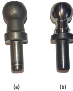
Fig.7 (a) Preform by cold forging, (b) final form by machining.
