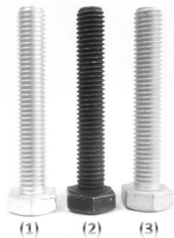
Figure 1. Bolt specimens coated with 1-) Zn Cr 3 + TnT 11, 2-) Delta-Protekt ® KL100 + Delta Seal GZ Black and 3-) Delta-Protekt ® KL100 + VH301 GZ.
