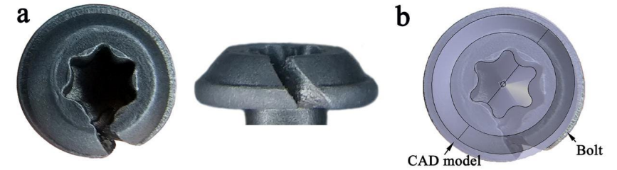
Figure 3. Crack evolution on the bolt; (a) top and front view and (b) comparison of the damaged bolt and CAD model.
